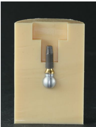
Fig. 14a: Implant positions in the embedding mold; Sectional view. Fig.
